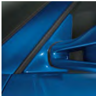
Mirror attachment point finishers painted
